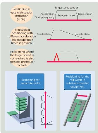
• The minimum startup time (i.e., the time between instruction execution and pulse output) is 46 µs, with an impressive 70 µs for trapezoidal acceleration/deceleration.
