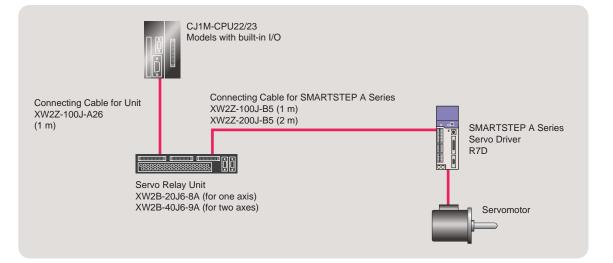
For connections other than those involving Servo Drivers and Servomotors, wire to terminal blocks using an XW2Z-DCK Connecting Cable and an XW2D-40G6 or XW2B-40G5/4 Connector Terminal Conversion Unit.
