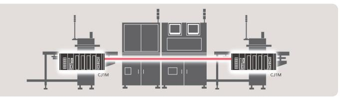
Data can be exchanged via Serial PLC Links involving up to nine CJ1M PLCs using the built-in RS-232C Boards. Up to ten words per PLC can be allocated to the Serial PLC Links. RS-232C can be converted to RS-422A easily using a CJ1W-CIF11 RS-422A Converter.
