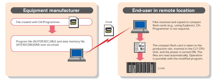
Programs can be written to a compact flash card without a PLC being present. The cards can be used with PC card slots, which are built into most laptop computers, and so special peripheral devices are not required.
