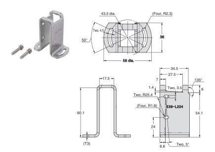
**Photoelectric Sensor** Accessory are installed (Example of E3AS-HL500□)
