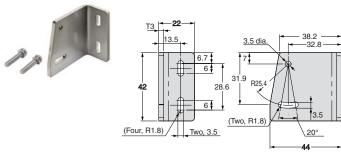
Photoelectric Sensor Accessory are installed (Example of E3AS-L200□)
