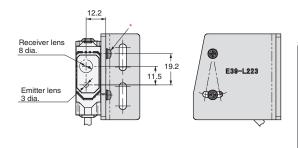
\* Accessories 2-M3-L10 Cross Recessed Pan Head Screws (Attached to SW+JIS W)
