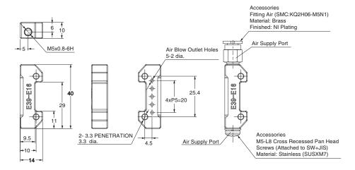
Photoelectric Sensor Accessory are installed (Example of E3AS-HL500□)
