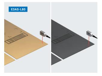
Detection may become unstable as differential travel varies depending on the workpiece color. The E3AS-L80 Sensor can reliably detect level difference regardless of color since its differential travel for black paper is 5%.
