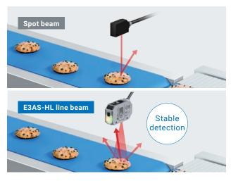
With spot beam, detection is unstable since the reflected light does not reach the sensor depending on the profile of the workpiece surface. With the line beam of the E3AS-HL Sensor, detection is less affected by the profile of the surface since the reflected light reaches the sensor from any part of the surface.
