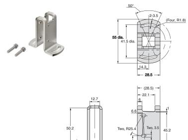
Photoelectric Sensor Accessory are installed (Example of E3AS-L200□)
