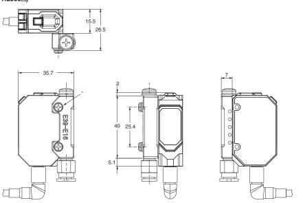
**Photoelectric Sensor** Accessory are installed (Example of E3AS-HL500□)
