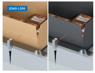
When the workpiece is low-reflective black paper, detection may become unstable due to insufficient sensing distance. The E3AS-L200 Sensor can stably detect at the same distance regardless of color since its sensing distance for both white paper and black paper is 200 mm.
